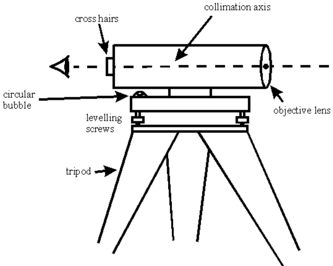
The level is mounted on a tripod, and has three levelling screws that (in conjunction with a circular bubble) allow the level to be levelled. These screws have a limited range and the tripod head must be set approximately level beforehand by adjusting the tripod legs.
