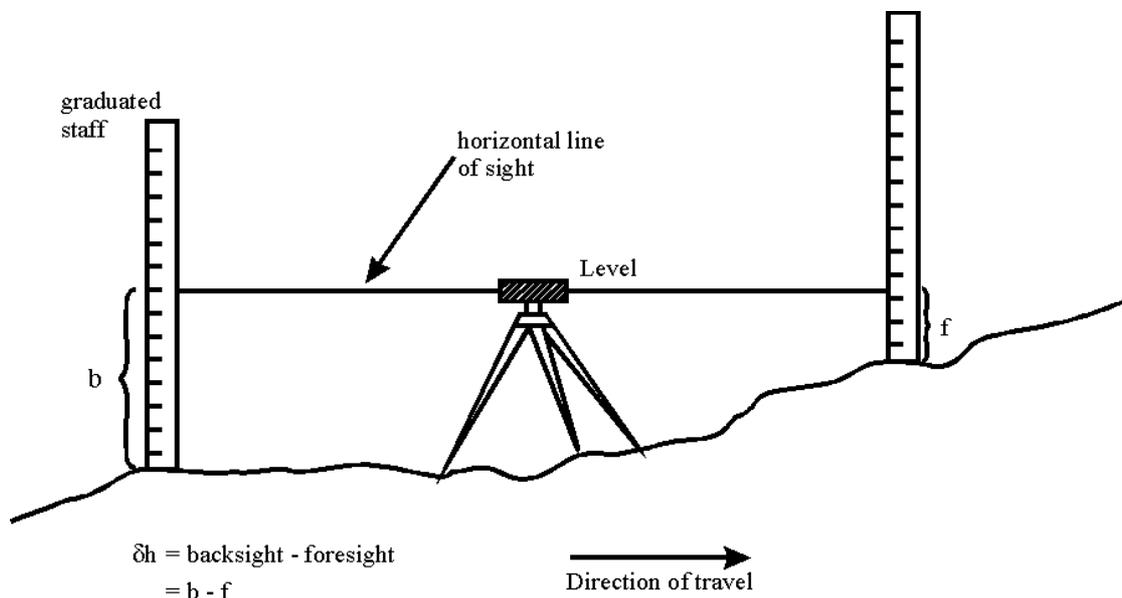
A graduated staff is held vertically over the first point and a reading made of the intersection of the cross-hair with the image of the staff (backsight - b). The same (or an identical) staff is then held vertically over the second point and a further reading made (foresight - f). The difference between the two readings is the difference in height between the two points:
